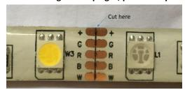
You can re-join the strip light with the 3pc connector which is included in the package
